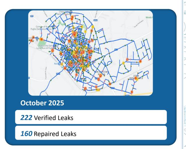
There has been a clear improvement and a significant reduction in the number of potential leaks and noise signals detected in the network. In particular, over the course of a year, 222 leaks were verified, and 160 were repaired, thanks to the deployment of noise loggers.
